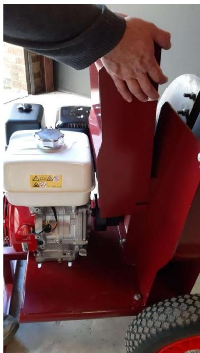
Remove the protective cover that sits over the belts with a 13mm socket.
