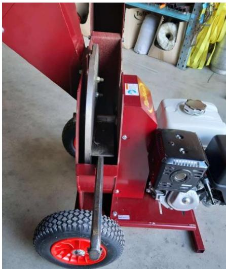
Open the discharge chute and place a bar between one of the flaps of the flywheel and the frame of the machine as shown. Ensure that the flywheel doesn't rotate when this bar is in place by pulling the engine cord.
