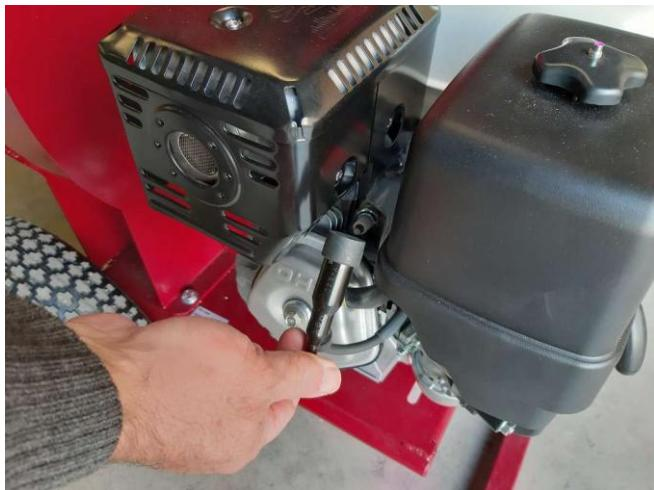
Disconnect the spark plug to ensure that the machine will not receive power whilst you are working on the flywheel
