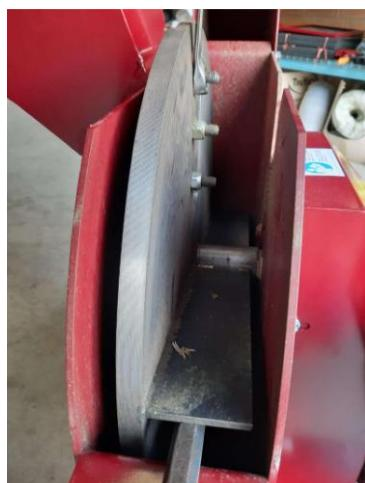
Using a 19mm spanner, loosen the nut and bolt that connects the chipper blade to the flywheel.
