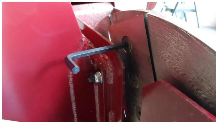
When retightening the nut and bolt, the rotation of the spanner will force the flywheel the opposite direction. Use the Allen key against the frame of the machine as pictured to prevent the flywheel from rotating whilst the nut is being tightened.
