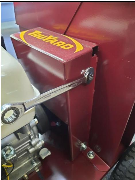
Remove the protective cover that sits over the belts with a 13mm socket.
