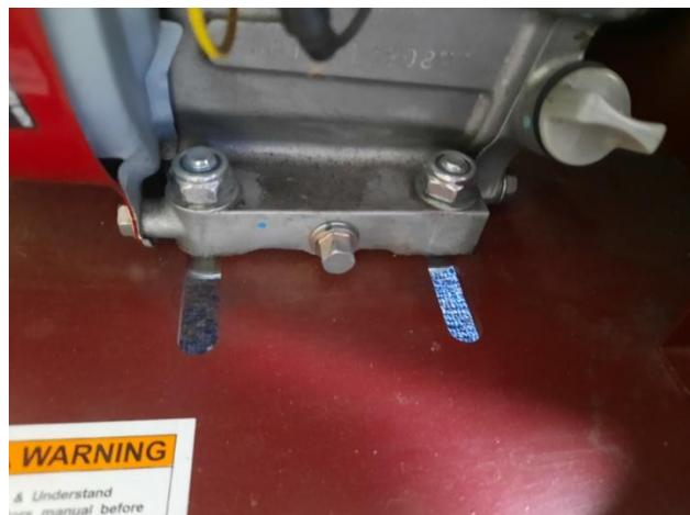
Using a 17mm spanner, loosen the nuts that connect the engine to the frame of the machine. Once all four have been loosened, slide the engine on the rails to increase the belt tension. Retighten the nuts and ensure that the engine is secure.
