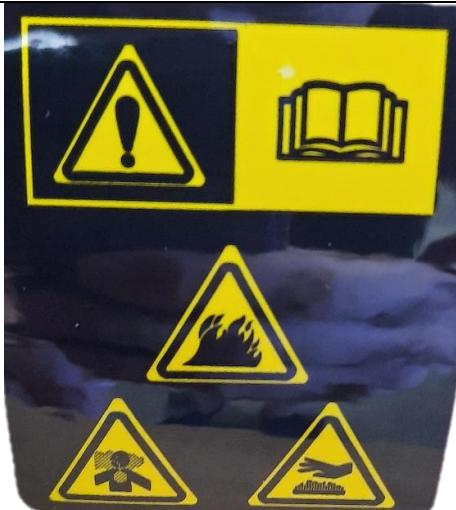
**CAUTION** – the operating of the engine, its maintenance and starting must be done after having read the manual to prevent any harmful incidents and misuse of the engine from occurring
