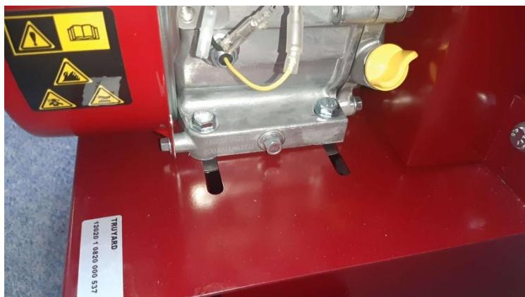
Using a 17mm spanner, loosen the nuts that connect the engine to the frame of the machine. Once all four have been loosened, slide the engine on the rails to increase the belt tension. Re-tighten the nuts and ensure that the engine is secure.
