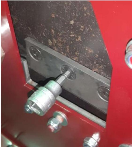
In order to fully remove the nut and bolt, use an 8mm Allen key to counter the force from the spanner. Remove the nuts and bolts from the chipper blade. Once all three have been removed, take out the chipper blade. When replacing the chipper blade, ensure that the flywheel does not move and that it is facing the correct direction.
