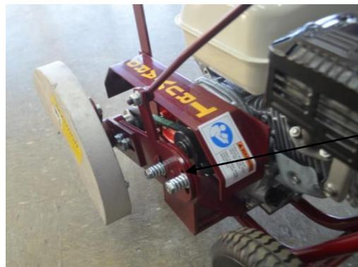
**WARNING:** Make sure the spark plug lead has been disconnected. Undo the two bolts on the blade flange. Pull the cutting head out so the belt is tight. Redo the bolts up. Do not over tighten drive belt
