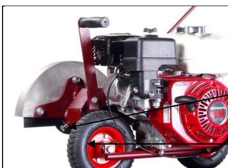
**WARNING:** Make sure the spark plug lead has been disconnected. The blade guard position can easily be adjusted by loosening the bolt under the guard. Move it to the desired position and re-tighten. Do not over inflate the pneumatic wheel. Maximum PSI is 18.
