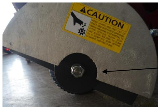
**WARNING:** Make sure the spark plug lead has been disconnected. Put a Stiltson on the pulley in the inside of the blade guard. Undo the bolt on the end of the drive shaft. It is best to use a air gun to remove this. Be careful the blade might rotate while loosening or tightening.
