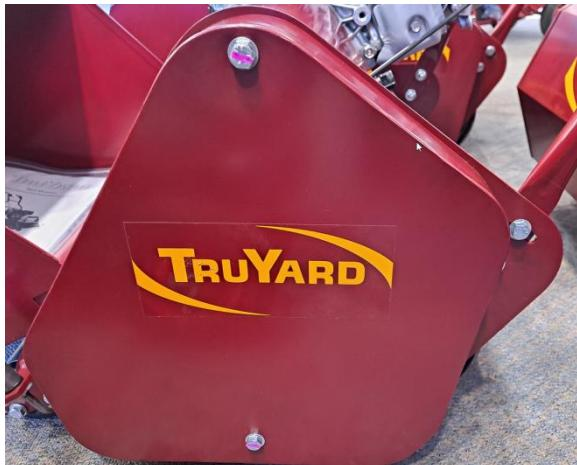
Remove the chain case cover on the side of the mower. Clean away any built up dirt and grass clippings. Lubricate with chain oil to increase the life of your chains.
