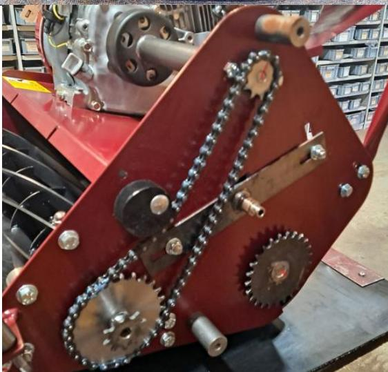
Check the chain tension. If loose, move the nylon adjuster to give the correct tension.
